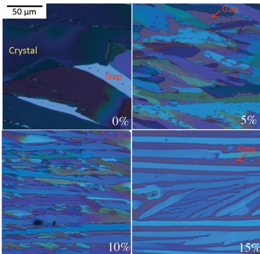
**Figure 3.** Polarized optical microscopy images of drop-cast TIPS pentacene films with  $\text{SiO}_2$  concentrations of 0%, 5%, 10%, and 15%. All images share the same scale bar, which is shown at the top left.
