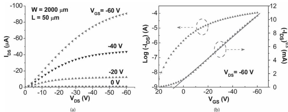
**Figure 1.** Typical output (left) and transfer characteristics (right) of SiO<sub>2</sub> nanoparticle/TIPS pentacene OTFTs. The shown device has a SiO<sub>2</sub> concentration of 10% by weight. The measured saturation mobility is 0.1 m<sup>2</sup> V<sup>-1</sup> s<sup>-1</sup>, with a threshold voltage of 8 V and on/off ratio above 10<sup>4</sup>.
