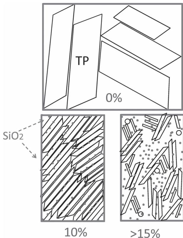
**Figure 7.** Sketches representing TIPS pentacene films with different SiO<sub>2</sub> nanoparticle concentration. “TP” stands for TIPS pentacene crystals.
